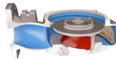
Stage 2. Solids slide along the tip of the impeller vane inside the relief groove. The guide pin in the insert ring pushes all types of solids away from the center of the impeller, along the leading edge and out through the relief groove.
